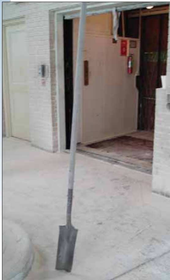
The 40-ft, 75-lb pole used to move the lime was difficult to use and contributed to personnel injuries and operations inefficiencies.
